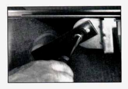
Remove the bolt from the engine cover bracket.
